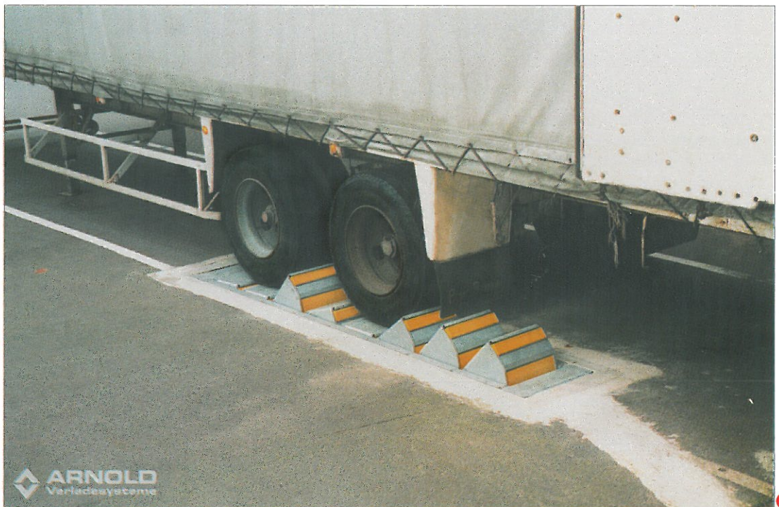
Truck with two axles stopped by ARS.
